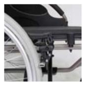
'Pull-to-lock' brake With folding lever for easier side (3) (3J) (4)
