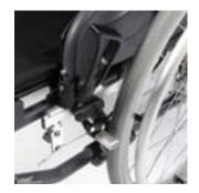
OAD wire-controlled brake Allows the user to brake the chair with one hand. (3)(4)
